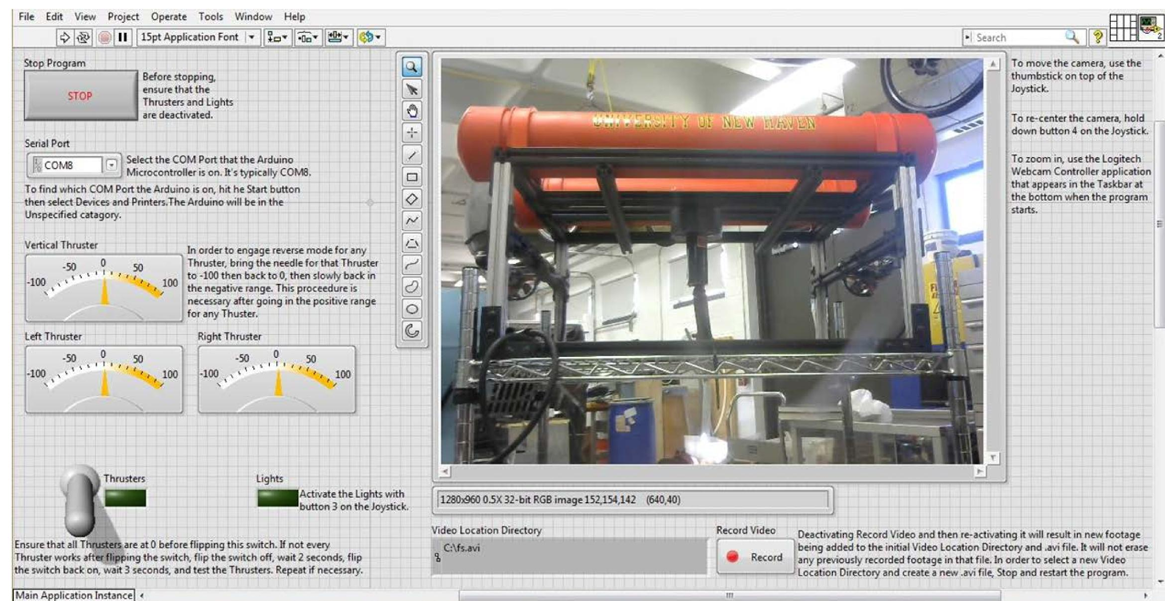
This is the LabVIEW Front Panel which serves as the user interface. It provides a display for live video from the onboard camera, thruster throttle and light indicators, and a recording control button. The operation instructions are also provided on the panel for easy reference.
