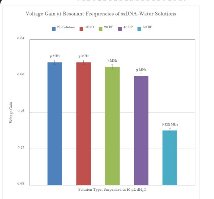
Same voltage gain trend as PBS solutions. DNA resonant frequency still undetermined to have any correlation to length of DNA strands, further studying will ensue.
