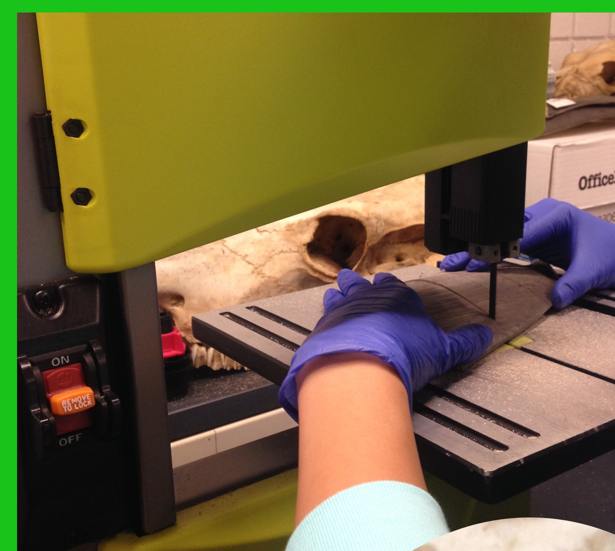
Figure 1: A band saw was used to slice the fins into percentages of 20, 40, 60 and 80.
