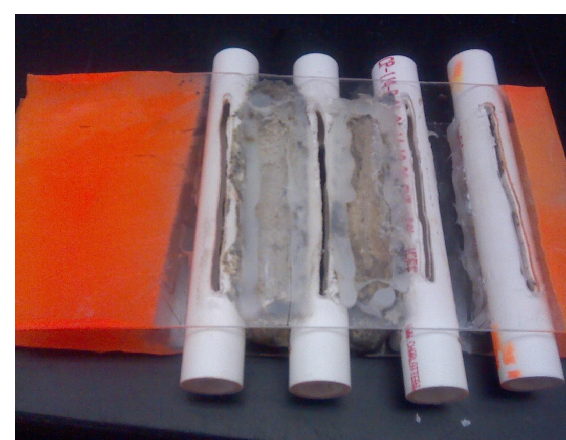
Figure 3. A picture of one of the pore water sampler (peeper) used during the experiment.
