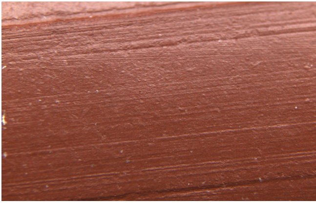
Figure 3. Land of fired .40 caliber bullet Mikrosil® cast at 35x magnification
