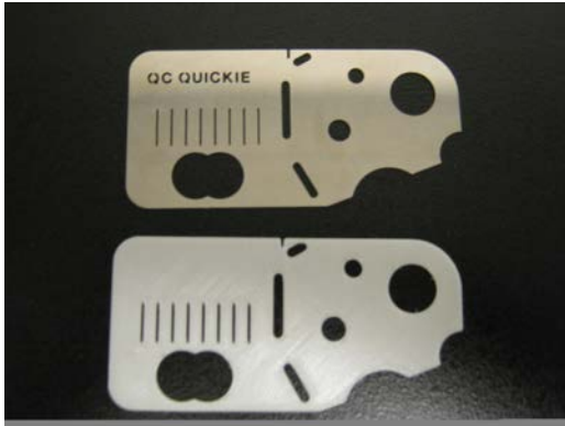
Figure 2. Original benchmark part (top) next to a replicated part from the uPrint 3D printer (bottom).
